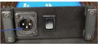
Figure 1-8 Connecting XLR to Direct Box
