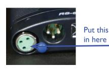
Figure I-50 Com Connection
