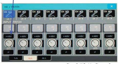
Figure 2-46 Enabling Phantom Power
